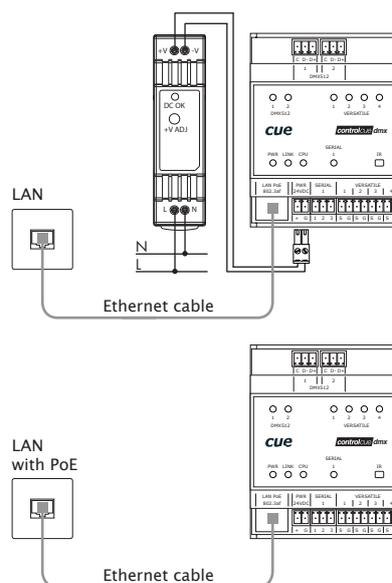
Delivered DIN rail power supply 24 VDC can be used for areas without PoE infrastructure.
